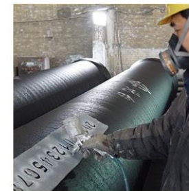
Finishing, mark painting
