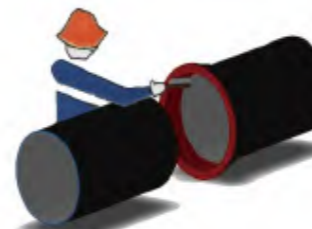
清理承口示意图 Schematic diagram of cleaning the socket
