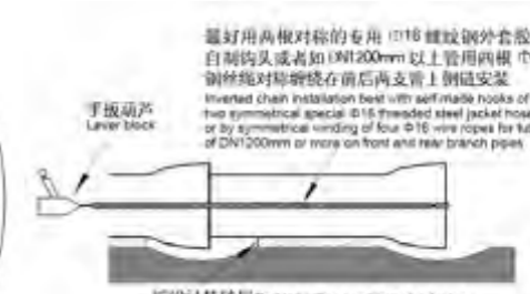
大口径安装示意图 Large caliber installation diagram
