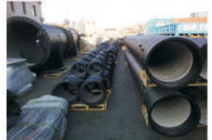
内衬水泥, 外锌+沥青漆管件 Internal coating cement, outer zinc layer and asphalt paint layer pipe fittings
