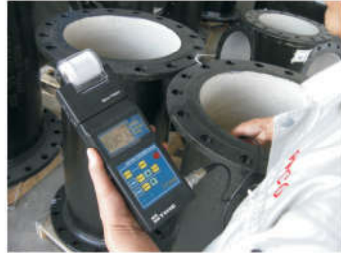
10. 覆层厚度检测 Lining thickness measure
